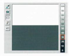
Using tools similar to a paint program, this BAM was created within LD2000 to allow 100% power for the top half of the projection area and 30% power for the lower half.
